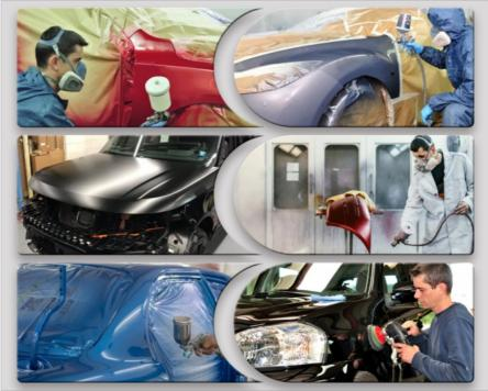
The shelf life of 1K red auto repair paint is generally about 12 months to 24 months, depending on the storage conditions and packaging methods. During storage, it should be avoided from direct sunlight, high temperature, humidity and other environments to avoid affecting the quality and performance of the paint. At the same time, the paint should be sealed to prevent solvent evaporation and air from entering.
